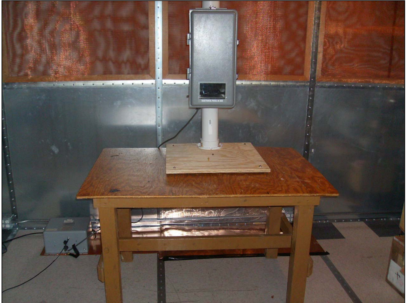
Photograph 1. Conducted Emissions, Test Setup
