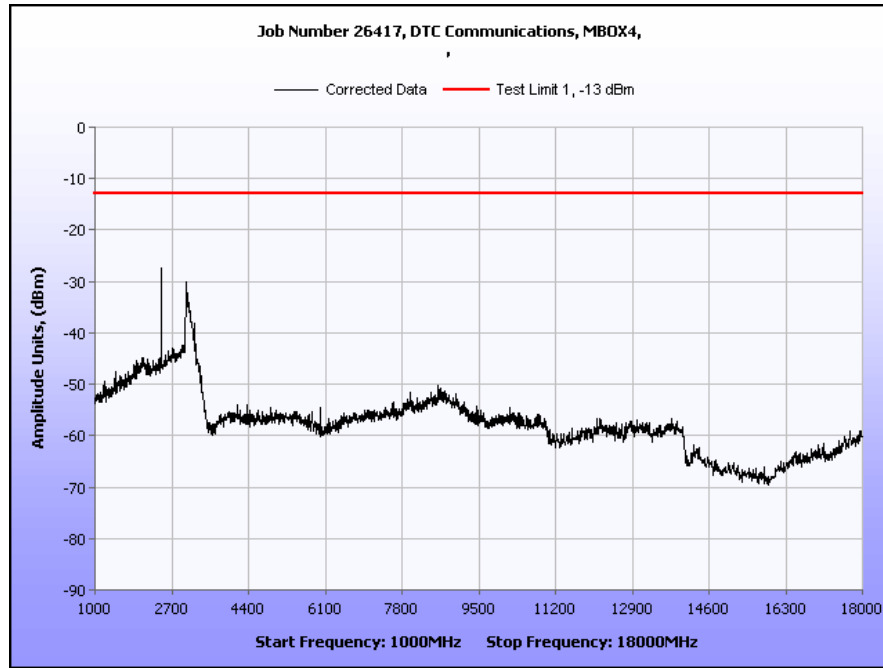
Plot 93. Radiated Spurious Emissions, Mid Channel, 8 MHz, 1 GHz – 18 GHz
