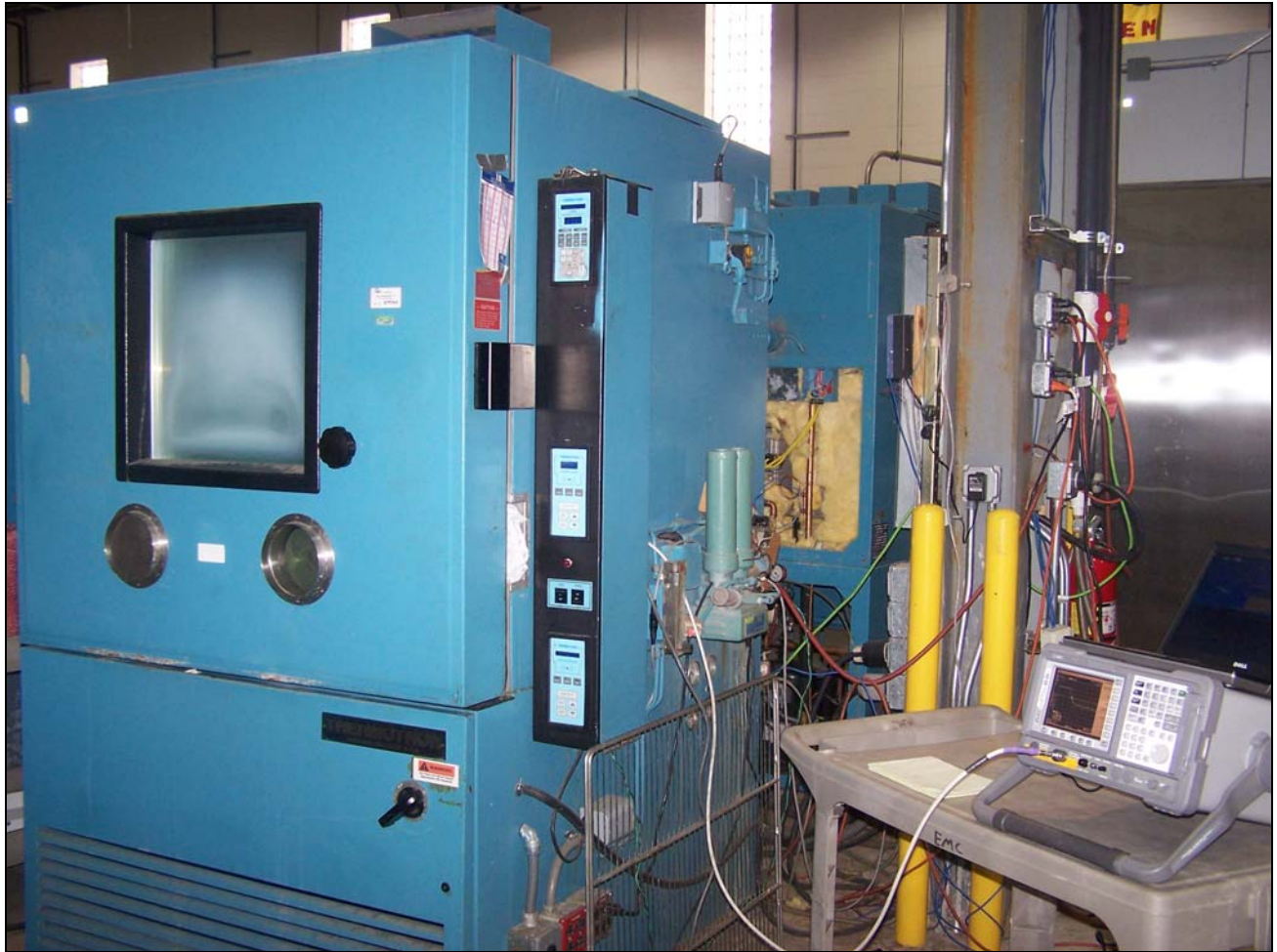
Photograph 4. Frequency Stability, Test Setup
