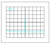
Figure Four: Position the calibration signal marker in the center as shown above. This will center the analyzer at 170 MHz
