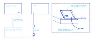
Confirm the 9 Volt battery in the LB-1A Final Test Fixture is new. Place the test housing on the UUT.
