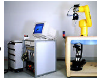
Fig. 1 SAR Test Setup
