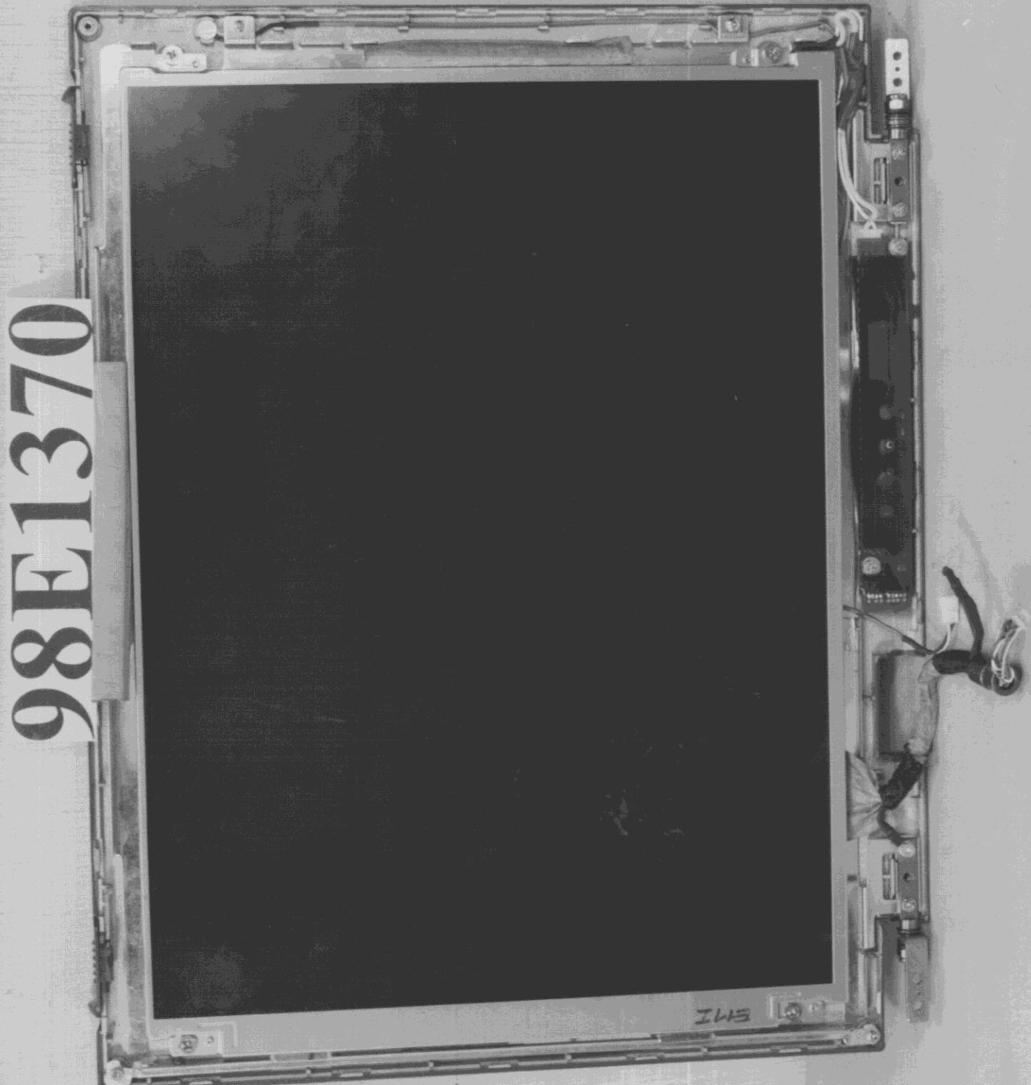
37. Photo # 37. 13.3" Panel Unit Partially Disassembled
