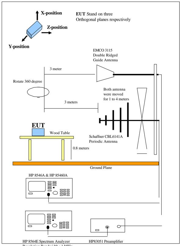
Resolution Bandwidth: 1 MHz Video Bandwidth: 1 MHz
