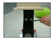
Step 3. Mount the Valve Handle Adaptor onto the "shaft" of VCM and screw tightly on the flat side of "shaft".
