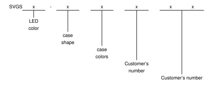
The case shape: such as right angle, concave, convex and special angle.
