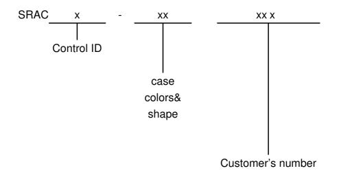
The case shape: such as right angle, concave, convex and special angle. The case shape will not influence PCB board.
