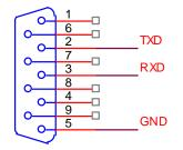
Pin2: TXD Pin3: RXD Pin5: GOUND Pin 1,4,5,6,7,8,9 : No Connection.
