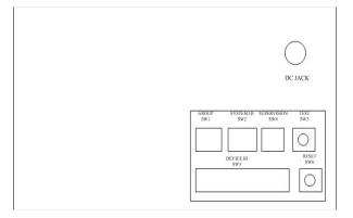
**SW 3 :** A 12-pin dip switch block to set the "Unit ID Number".
