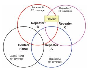
From the displayed diagram, the device is located between the RF coverage areas of Repeater B and C. Users can choose to learn the device into Repeater B only, learn into Repeater C only, or learn into both Repeaters B and C.
