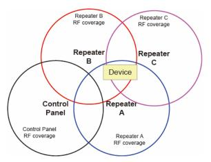
From the displayed diagram, the device is located between the RF coverage areas of Repeater A, B and C. Users can choose to learn the device into Repeater A only, learn into Repeater B only, learn into Repeater C only, or learn into Repeaters A, B and C.
