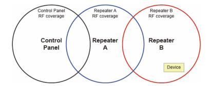
2. If a device is located between the RF coverage of multiple repeaters and the Control Panel:
