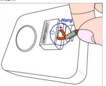
Step 2 Insert the cord into the opening of the fixture.
