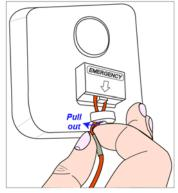
**Step 2** Release the hanging loop from the pull cord switch.
