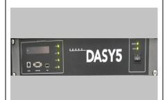
The DASY5 measurement server is based on a PC/104 CPU board with a 166MHz low-power Pentium, 32MB chip disk and 64MB RAM. The necessary circuits for communication with either the DAE4 electronic box as well as the 16-bit AD-converter system for optical detection and digital I/O interface are contained on the DASY5 I/O-board, which is directly connected to the PC/104 bus of the CPU board.
