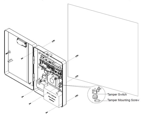
**Step 3.** Use the provided wall plugs for plaster/brick installation. Make sure the wall plugs are flush with the wall.
