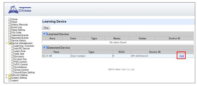
**Step 6.** If the device is successfully learnt into the system, the added device will be displayed in the "**Learned Device**" section.
