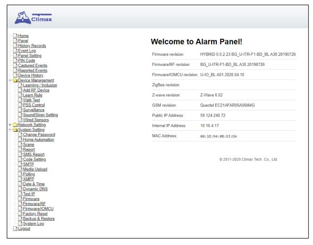
The Welcome page displays current control panel firmware version information according to different panel model and MAC address.
