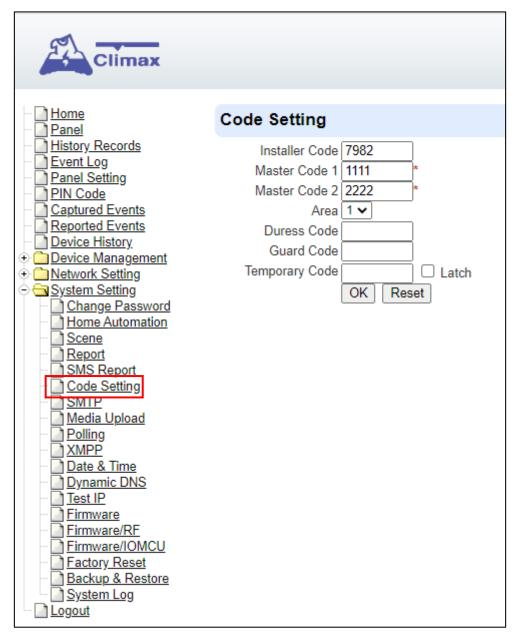
**Step 2.** You can also choose to have Latch Option On / Off for Temporary Code by tick the Latch Option box and press **OK** to confirm the settings.
