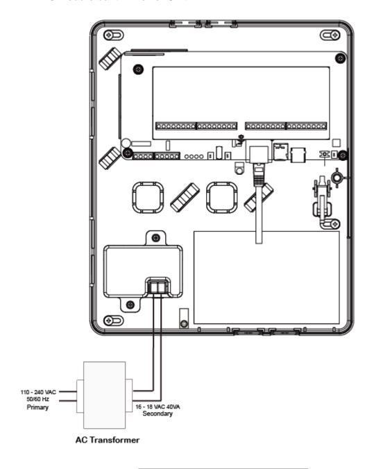
AC Module Built-in Power Unit: Connecting 2 wires of AC Transformer to 2 terminals of the Built-in Power Unit
