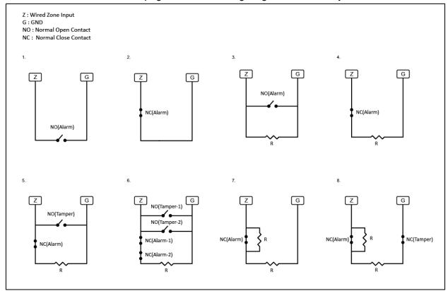
• **Resistor**: Select the resistance for the zone wiring.
