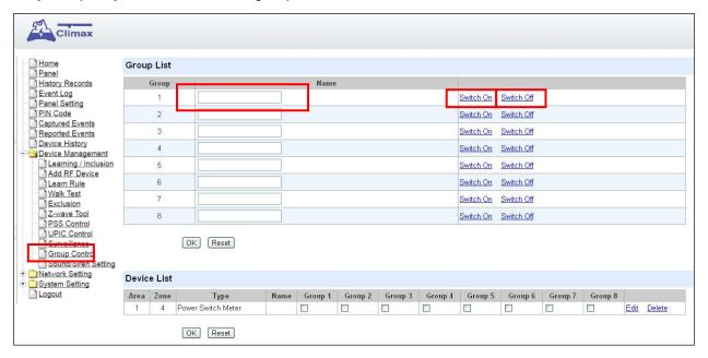
**Step 2.** Click Switch On or Switch Off to turn on or off one group of power switches.
