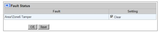
The fault events that exist in the alarm system are displayed under this section. When fault event exists in system, the control panel Fault LED will light up to indicate fault status under Disarm or Home Arm mode (The Fault LED will not light up under Arm mode).
