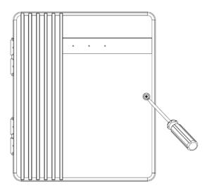
Step 2. Use the 4 mounting holes as a template to mark and drill holes appropriately.
