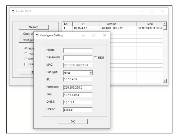
The LanType is default to **DHCP** and does not require manual input of IP/Netmask/Gateawy/DNS setting. If you wish to configure these setting manually, change LanType to **Static**.
