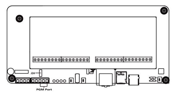
The PGM port can be a voltage output port or a dry contact relay output depending on J24 jumper settings.
