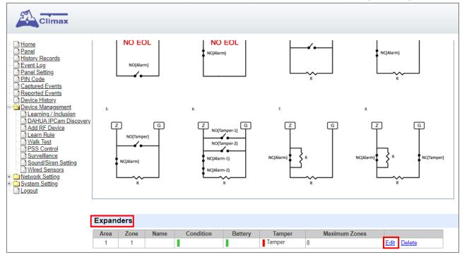
Step 3. Edit the type of the wired sensor, zone wiring, and the EOL resistance for each zone.
