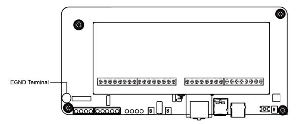
Using an insulated green wire (minimum 22 AWG), connect the EGND terminal and the grounding wire from the building electrical installation.
