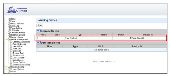
**Step 7.** Repeat Step 3~5 to learn in all device, click Stop to exit learn mode when complete. The system will automatically exit Learn mode if left idle for 5 minutes.
