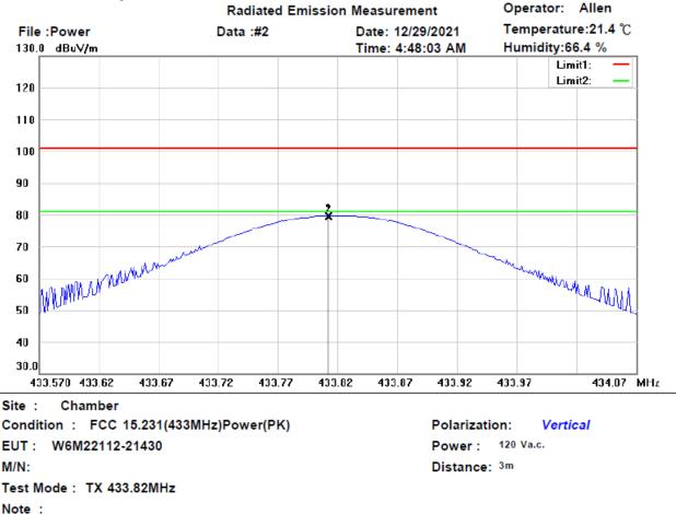
Reading Corr. factor Ant.Pos Tab.Pos Result Limit Margin Comment Detector Frequency Mk. (dB/m) (dBuV/m) (dBuV/m) (MHz) (dBuV) (cm) (deg.) (dB) 433.8125 54.72 peak 24.92 79.64 100.80 150 340 -21.16 433.8125 54.38 AVG 24.92 79.30 80.80 150 340 -1.50
