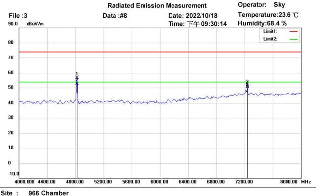
Condition : FCC\_part 15 RE-Class B\_Above 1GHz\_PK EUT : W6M22207-21977 M/N: Test Mode : Zigbee+WiFi
