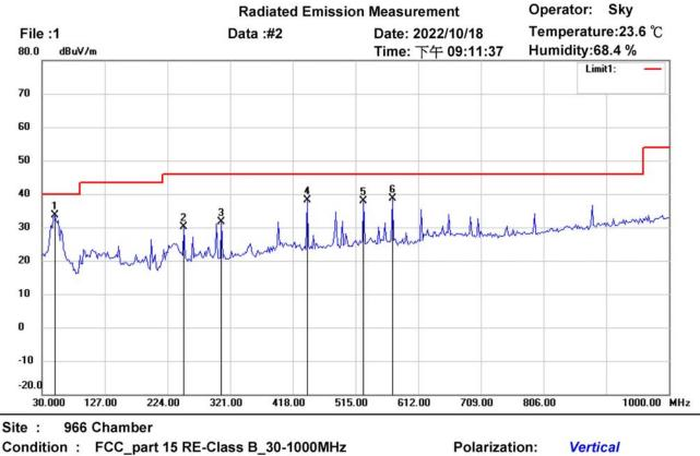
Condition : FCC\_part 15 RE-Class B\_30-1000MHz EUT : W6M22207-21977 M/N: Test Mode : Zigbee+WiFi
