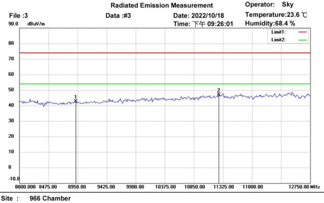
Condition : FCC\_part 15 RE-Class B\_Above 1GHz\_PK EUT : W6M22207-21977 M/N: Polarization: *Horizontal* Power : 120 Va.c. Distance: <sup>3m</sup>
