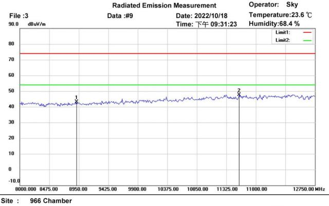
Condition : FCC\_part 15 RE-Class B\_Above 1GHz\_PK EUT : W6M22207-21977 M/N: Toot Mode : Zighee+WiEi Polarization: Vertical Power : 120 Va.c. Distance: <sup>3m</sup>
