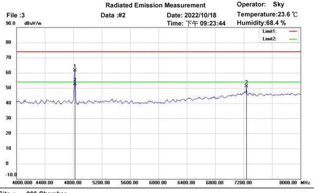
Site : 966 Chamber Condition : FCC\_part 15 RE-Class B\_Above 1GHz\_PK EUT : W6M22207-21977 M/N: Test Mode : Zigbee+WiFi
