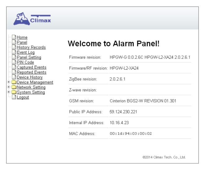
The Welcome page displays current control panel firmware version information according to different panel model and MAC address.
