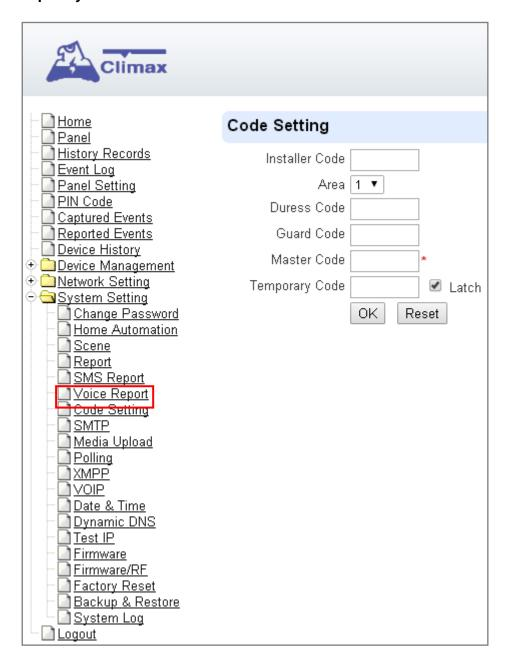
**Step 2.** You can also choose to have Latch Option On / Off for Temporary Code by tick the Latch Option box and press **OK** to confirm the settings.
