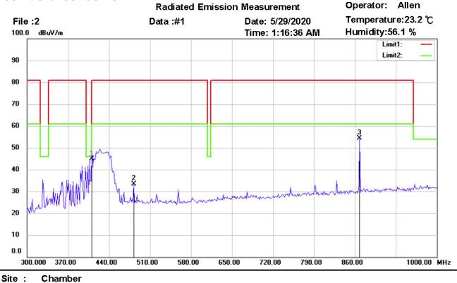
Condition : FCC 15.231(433MHz) 300-1000(PK) EUT : W6M22003-19782 M/N: Test Mode : TX 433.82MHz Polarization: Horizontal Power: 120 Va.c. Distance: <sup>3m</sup>
