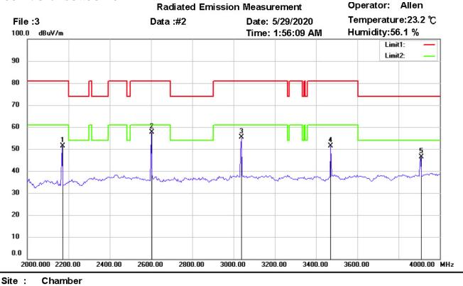
Condition : FCC 15.231(433MHz) 2000-4000(PK) EUT : W6M22003-19782 M/N: Test Mode : TX 433.82MHz Polarization: *Horizontal* Power : <sup>120</sup> Va.c. Distance: <sup>3m</sup>
