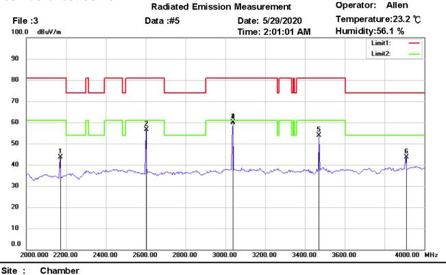
Condition : FCC 15.231(433MHz) 2000-4000(PK) EUT : W6M22003-19782 M/N: Test Mode : TX 433.82MHz Note : Polarization: Vertical Power : 120 Va.c. Distance: <sup>3m</sup>
