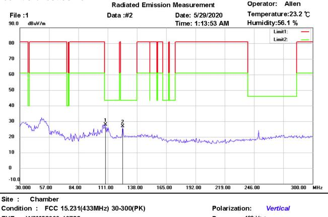
EUT: W6M22003-19782 M/N: Polarization: Vertica Power: 120 Va.c. Distance: <sup>3m</sup>
