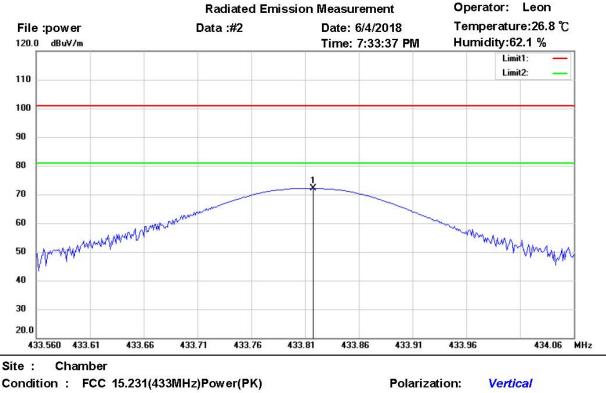
EUT : W6R21805-18133 M/N: Test Mode : TX 433.82MHz Note : Polarization: Vertical Power : 120 Va.c. Distance: 3m
