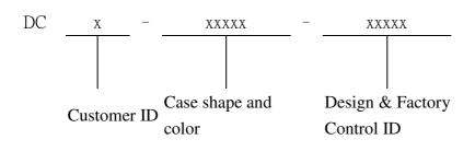
The case shape: such as right angle, concave, convex and special angle. The case shape will not influence PCB board.
