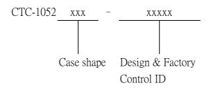
The case shape: such as right angle, concave, convex and special angle. The case shape will not influence PCB board.
