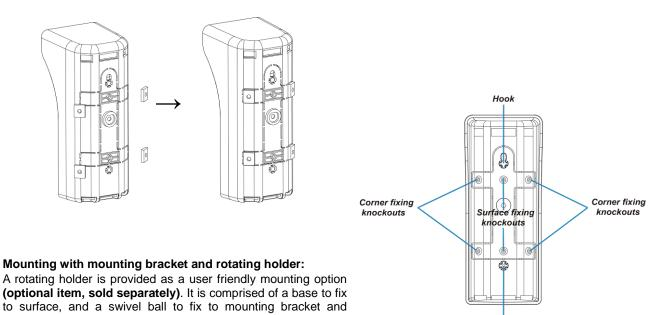
862EX. With the rotating holder, the PIR Camera can be rotated horizontally to provide optimal coverage.
