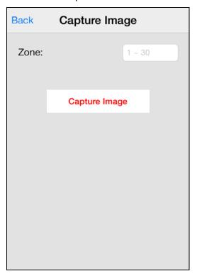
Specify the zone number of the PIR Camera you want to take picture, then press "Capture Image." A SMS message edit screen will appear for you to confirm. Press "Send" to send the SMS command to panel.
