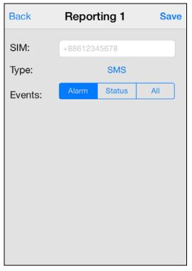
Enter the telephone number for reporting, and select report type and events. Only SMS(CID)/ SMS(Text)/ GSM CID/ Voice reporting options are available.  Press "Save". A SMS message edit screen will appear for you to confirm. Press "Send" to send the SMS command to panel.
