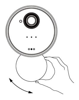
When adjusting the angle of the camera, make sure to keep the camera lens on the top for proper video recording.
