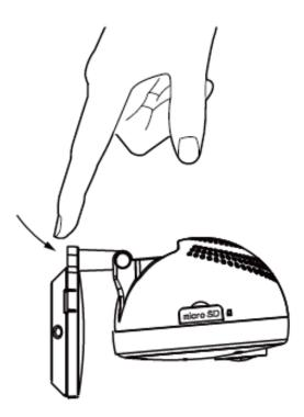
Make sure the three mounting hooks match the three latches on the mounting base before removal to avoid damaging the camera.
