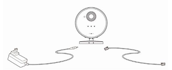
Step 2. Press and hold the Privacy Button and plug in the 5V DC power adapter.
