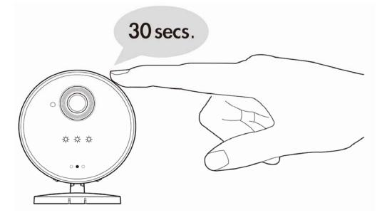
**Step 4.** When all 3 LEDs flash 3 times simultaneously followed by complete dimming of all LEDs, let go of the "Privacy Button".
