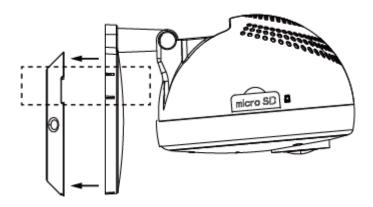
Step 5. Attach the Camera Stand onto the Mounting Base.
