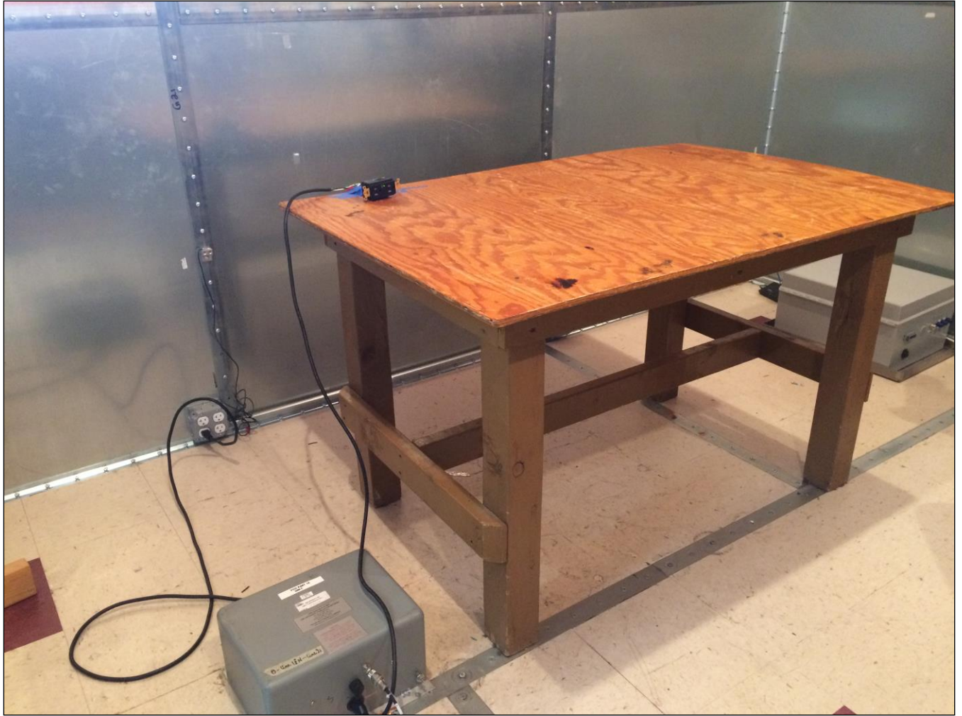
Photograph 1. Conducted Emissions, 15.207(a), Test Setup
