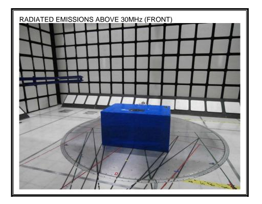
Note: The Log periodic antenna was taken as a representative test photo however a biconical was also utilized for testing as well which is not shown in set up photo.
