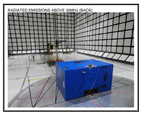
Note: The Log periodic antenna was taken as a representative test photo however a biconical was also utilized for testing as well which is not shown in set up photo.
