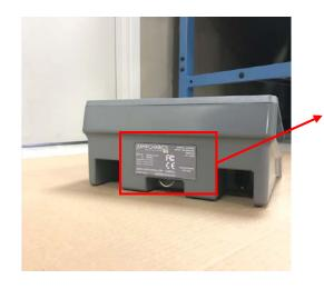
Label located on rear of JCEMDS unit on center of base
