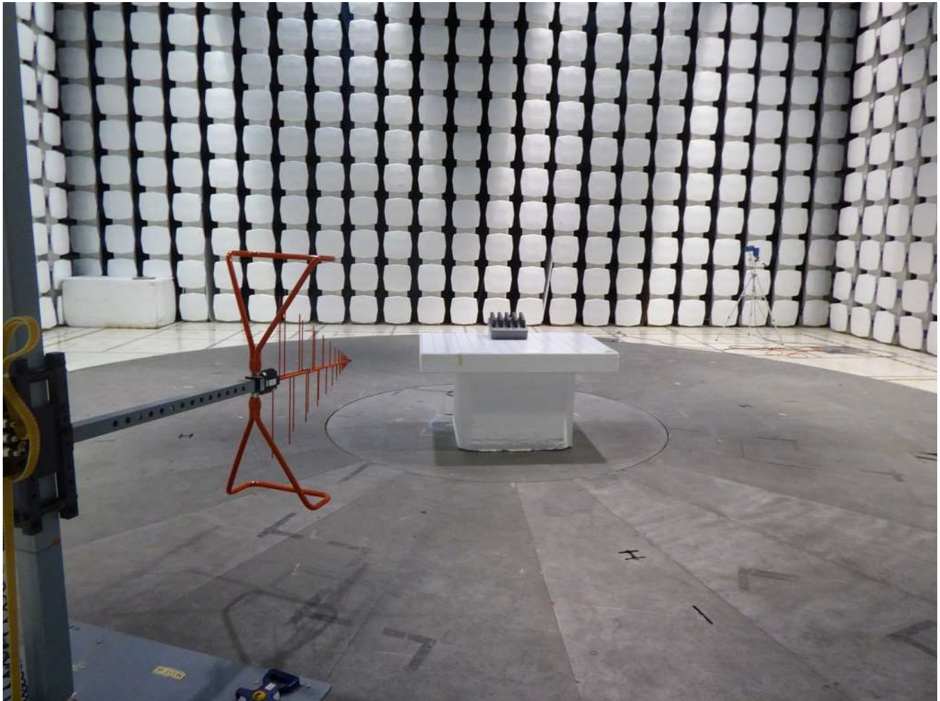
Figure 15 - Radiated Emissions Test Setup (30 – 1000 MHz, Charging)
