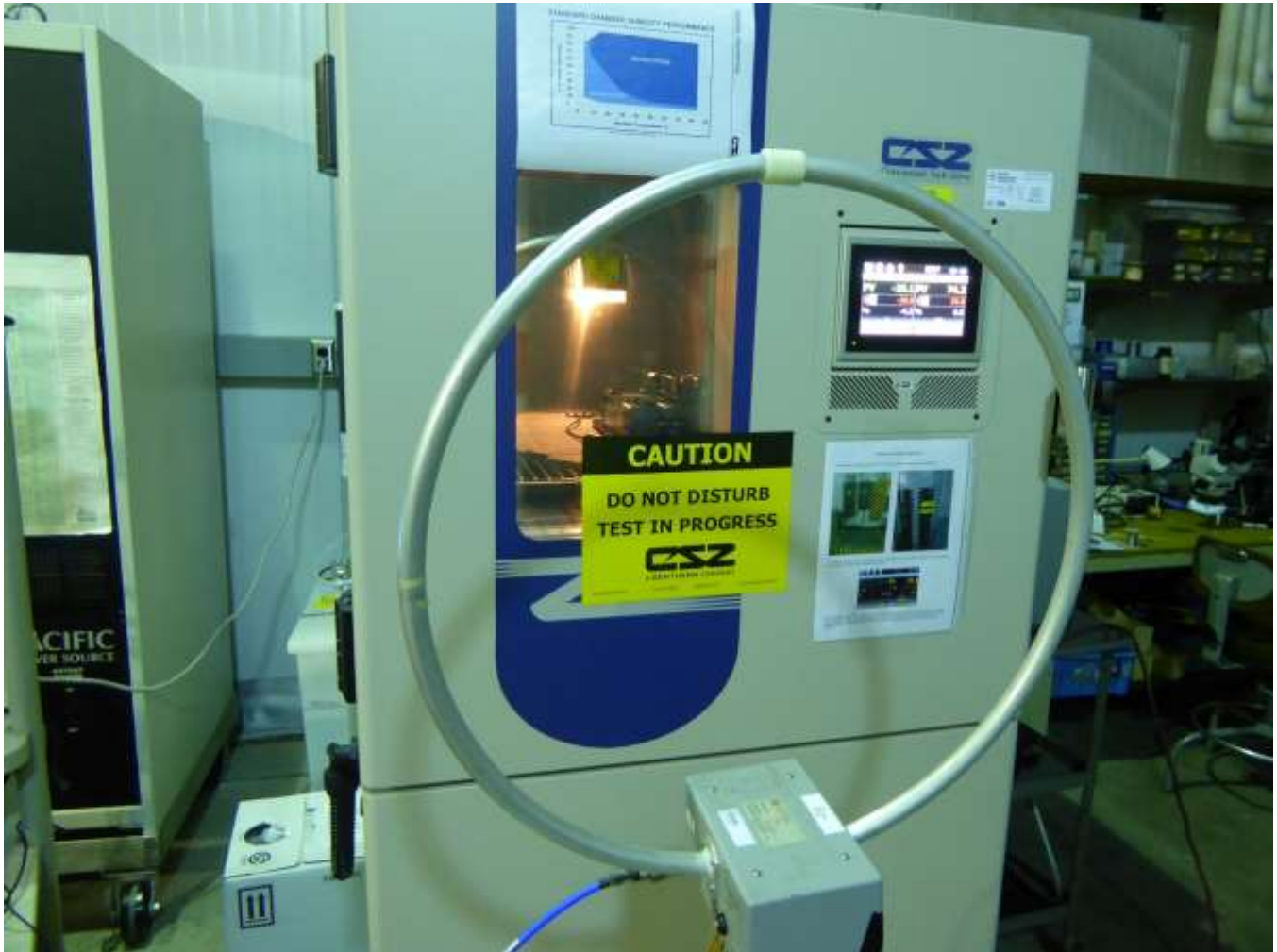
Figure 17 – NFC Frequency Stability Test Setup
