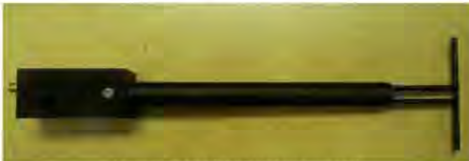
Figure 1 – MVG COMOSAR Validation Dipole
