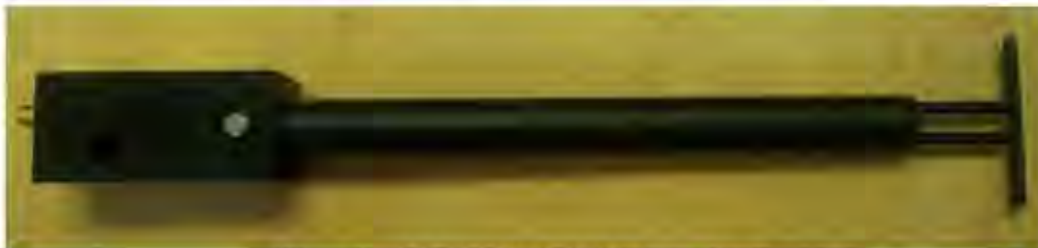
Figure 1 – MVG COMOSAR Validation Dipole
