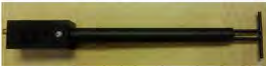
Figure 1 – MVG COMOSAR Validation Dipole
