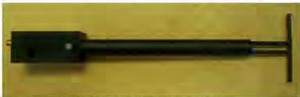
Figure 1 – MVG COMOSAR Validation Dipole
