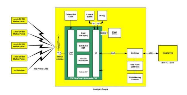
EUT is a <u>USB Receiver by Bluetooth Technology</u> with <u>79</u> channels. This device provided of transmitting speed <u>1~3Mbps</u>. The device of RF modulation is GFSK,  $\pi$  /4-DQPSK or 8-DPSK. The device adapts Frequency Hopping Spread Spectrum (FHSS). An embedded system can become Bluetooth enabled by inserting the Bluetooth RF module that interfaces to the embedded processor via USB interface.
