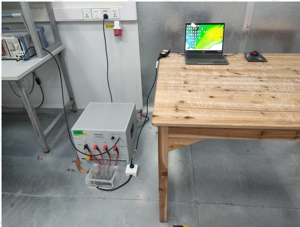
Photo of Conducted Emission Measurement
