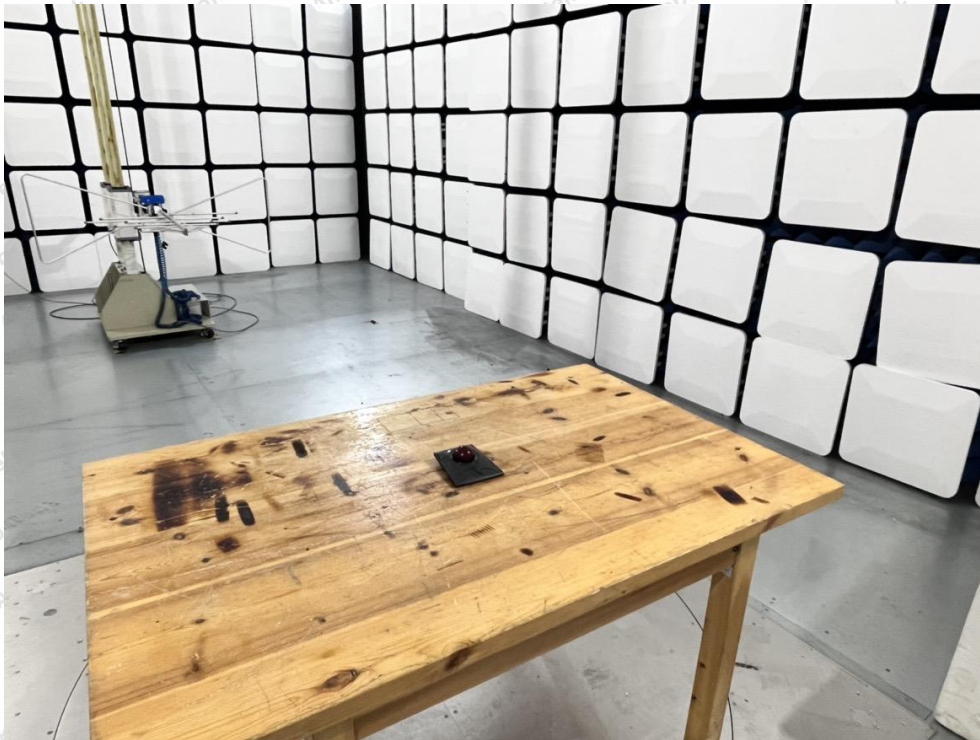
Photo of Radiation Emission Test
