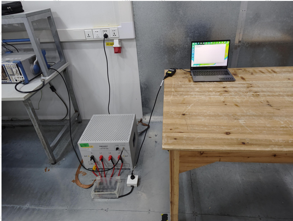
Photo of Conducted Emission Measurement
