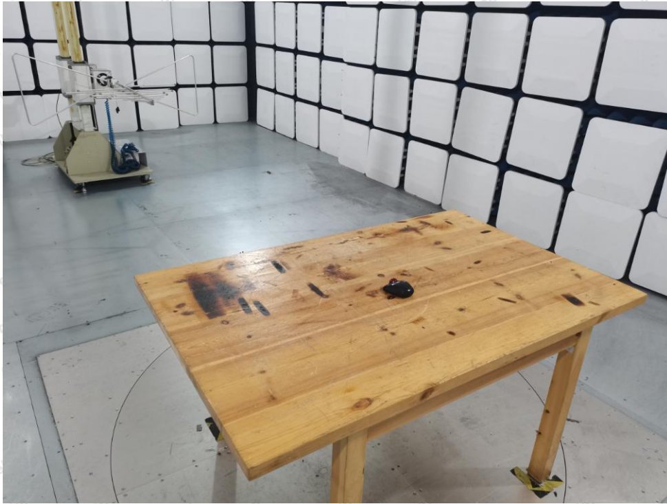
Photo of Radiation Emission Test
