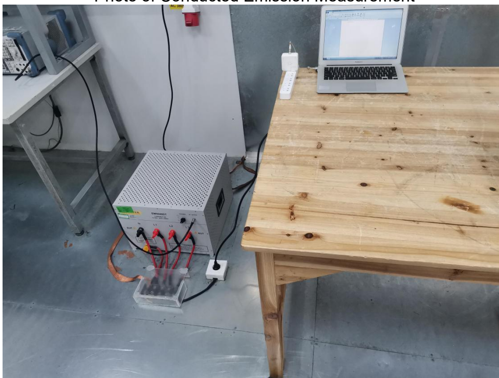
FCC ID:GV3M01592-D Photo of Conducted Emission Measurement
