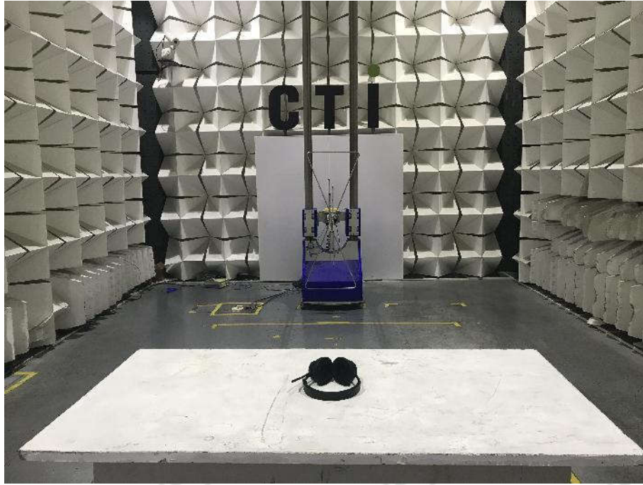
Radiated spurious emission Test Setup-1(Below 1GHz)
