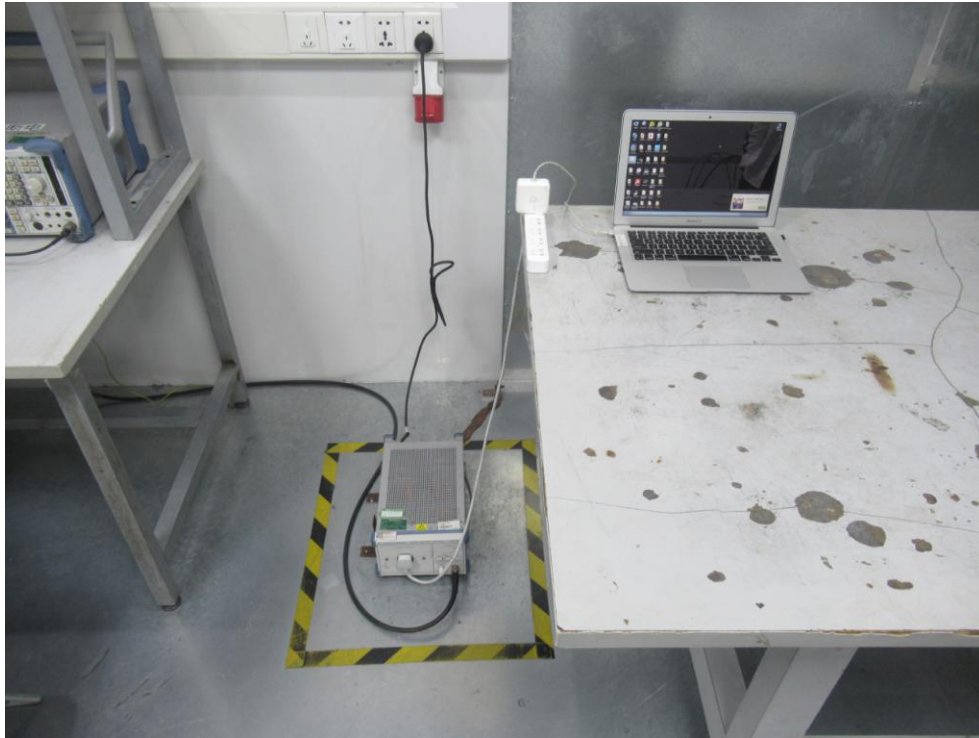
Photo of Radiation Emission Test
