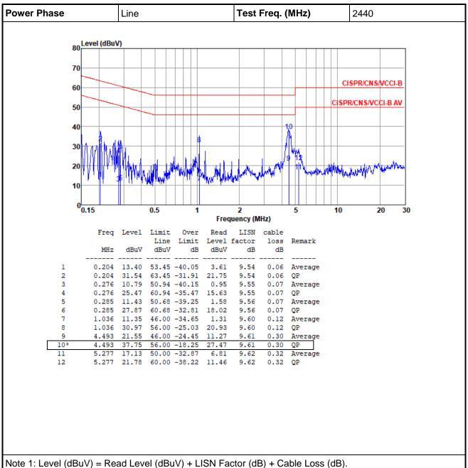
2: Over Limit (dB) = Level (dBuV) - Limit Line (dBuV).
