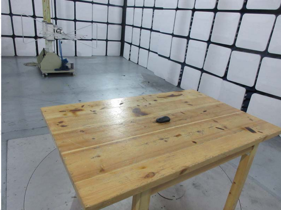
Photo of Radiation Emission Test
