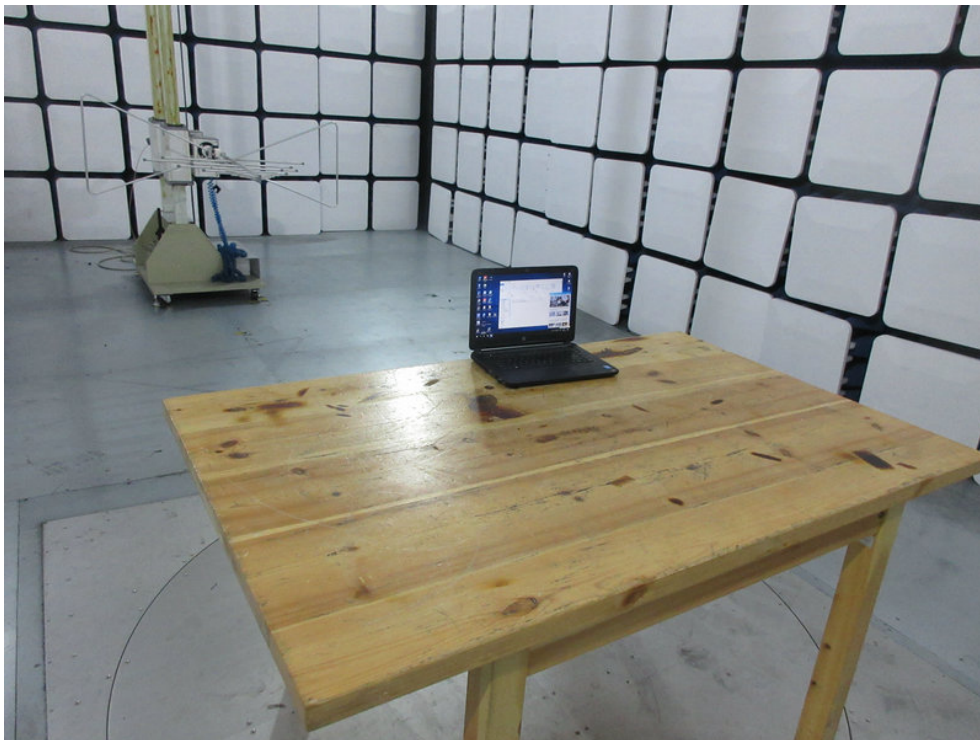
Photo of Radiation Emission Test
