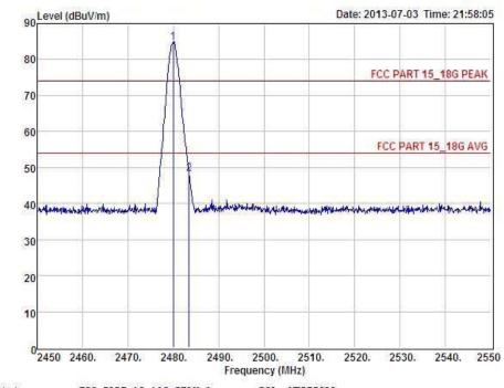
Condition : FCC PART 15\_18G PEAK 3m POL: VERTICAL : BLUETOOTH KEYBOARD : M01242 EUT
