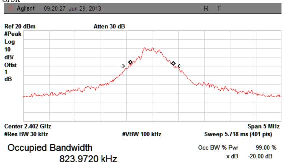
Transmit Freq Error -10.620 kHz x dB Bandwidth 858.450 kHz
