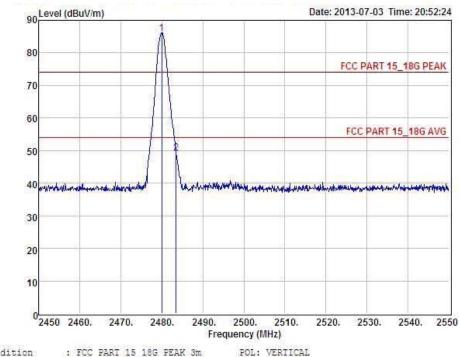
Condition : FCC PART 15\_18G PEAK 3m : BLUETOOTH KEYBOARD : M01242 : GFSK IX 2480MHz EUT
