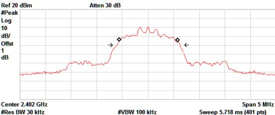
Occupied Bandwidth 1.1399 MHz Occ BW % Pwr 99.00 % -20.00 dB x dB
