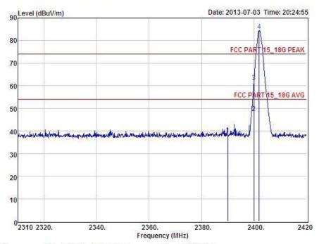
: FCC PART 15\_18G PEAK 3m : BLUETOOTH KEYBOARD Condition POL: HORIZONTAL
