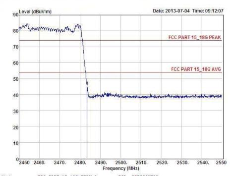
: FCC PART 15\_18G PEAK 3m : BLUETOOTH KEYBOARD Condition POL: HORIZONTAL
