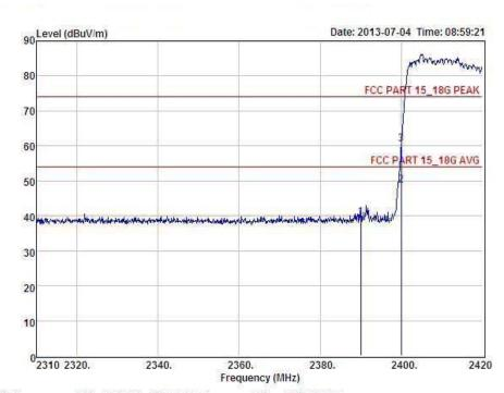
: FCC PART 15\_18G PEAK 3m : BLUETOOTH KEYBOARD POL: HORIZONTAL Condition
