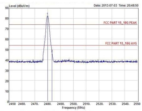
: FCC PART 15\_18G PEAK 3m POL: VERTICAL Condition EUT
