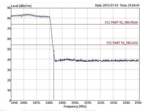
Condition : FCC PART 15\_18G PEAK 3m POL: VERTICAL EUT : BLUETOOTH KEYBOARD
