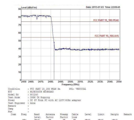
Remark: Level = Read Level + Antenna Factor - Preamp Factor + Cable Loss
