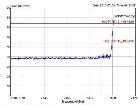
: FCC PART 15\_18G PEAK 3m : BLUETOOTH KEYBOARD Condition POL: VERTICAL
