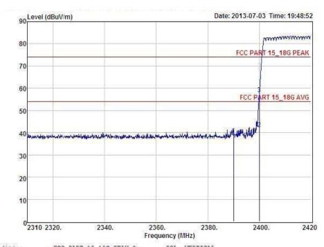
: FCC PART 15\_18G PEAK 3m : BLUETOOTH KEYBOARD Condition POL: VERTICAL
