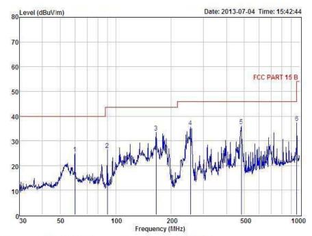
: FCC PART 15 B : BLUETOOTH KEYBOARD Condition POL: HORIZONTAL 3m
