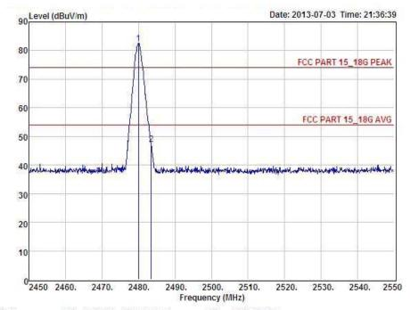
: FCC PART 15\_18G PEAK 3m : BLUETOOTH KEYBOARD POL: HORIZONTAL Condition
