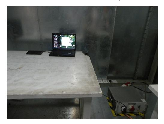
Radiated Emission Test Setup in Chamber
