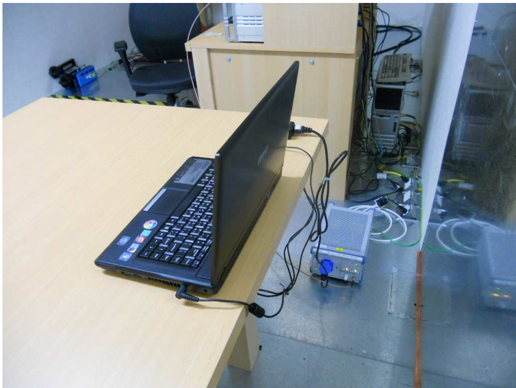
Photograph 4: Set-up for Mains Conducted Emissions (Back View)
