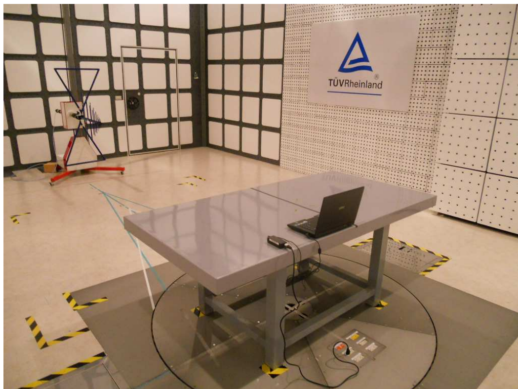
Photograph 2: Set-up for Spurious Emissions (Back View)
