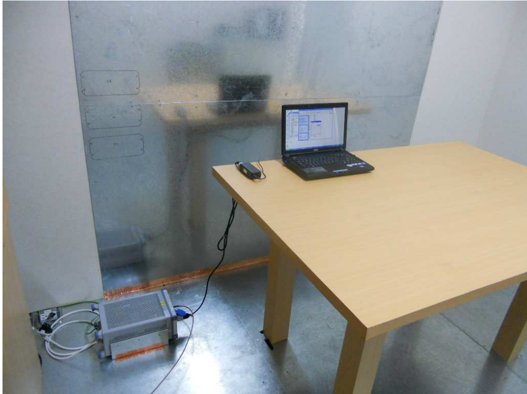
Photograph 4: Set-up for Mains Conducted Emissions (Back View)
