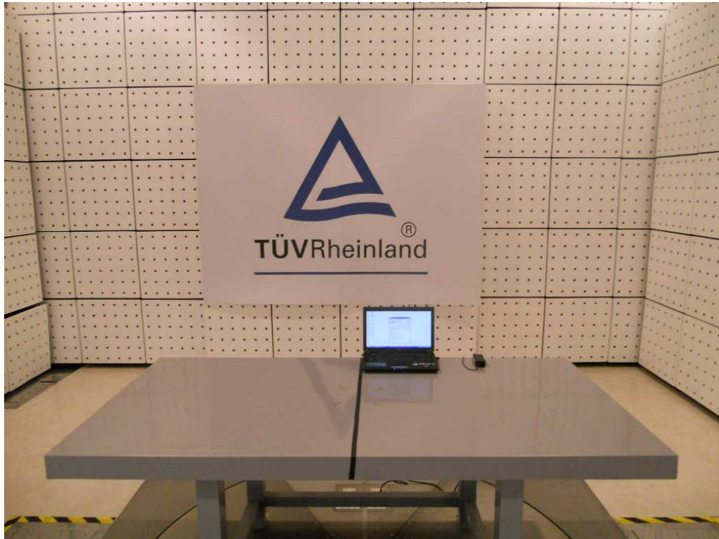
Photograph 2: Set-up for Spurious Emissions (Back View)
