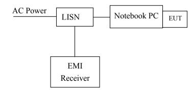
The EUT are connected to the main power through a line impedance stabilization network (LISN). This provides a 50 ohm/50uH coupling impedance for the measuring equipment. The peripheral devices are also connected to the main power through a LISN that provides a 50ohm/50uH coupling impedance with 50ohm termination.
