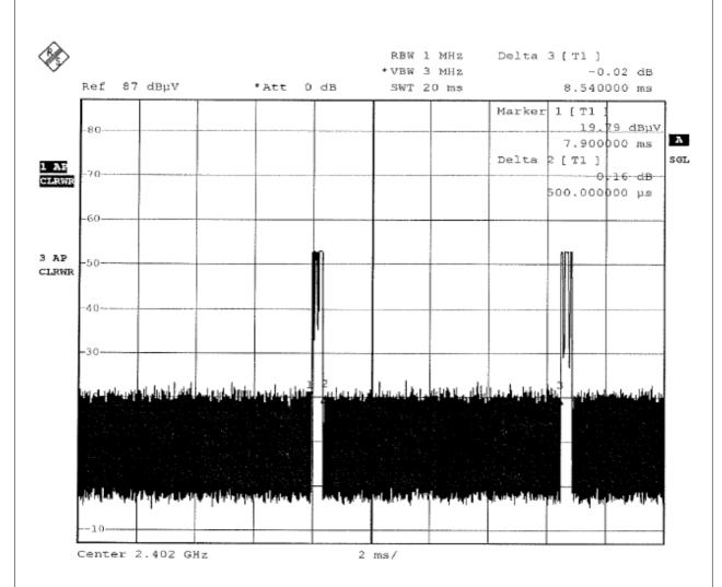
$$20\log(\text{Duty cycle}) = 20\log\frac{0.5 \text{ ms}}{8.54 \text{ ms}} = -24.65 \text{dB}$$
