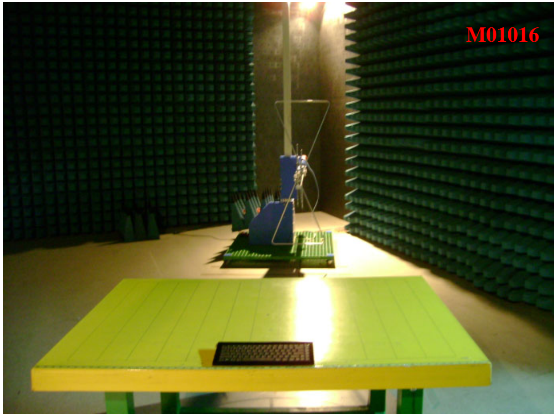
Photo 1: Radiated Emission Test set-up photo
