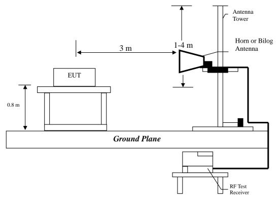
The frequency range from 30MHz to 1000MHz using Bilog Antenna. The frequency range over 1GHz using Horn Antenna.
