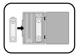
Install batteries at the bottom of the mouse
