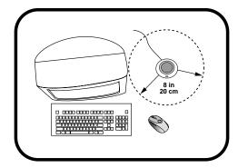
Place the wireless receiver at least 8 inches away from other electronic devices. Wireless range is about 6 feet between the mouse and the receiver.
