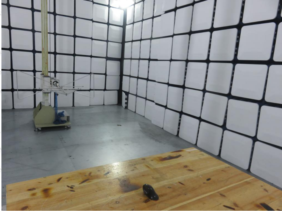
Photo of Radiation Emission Test
