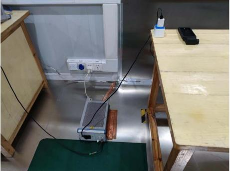
1.2 Photograph – Radiated Emissions Test Setup For 9KHz-30MHz Test Site 1#
