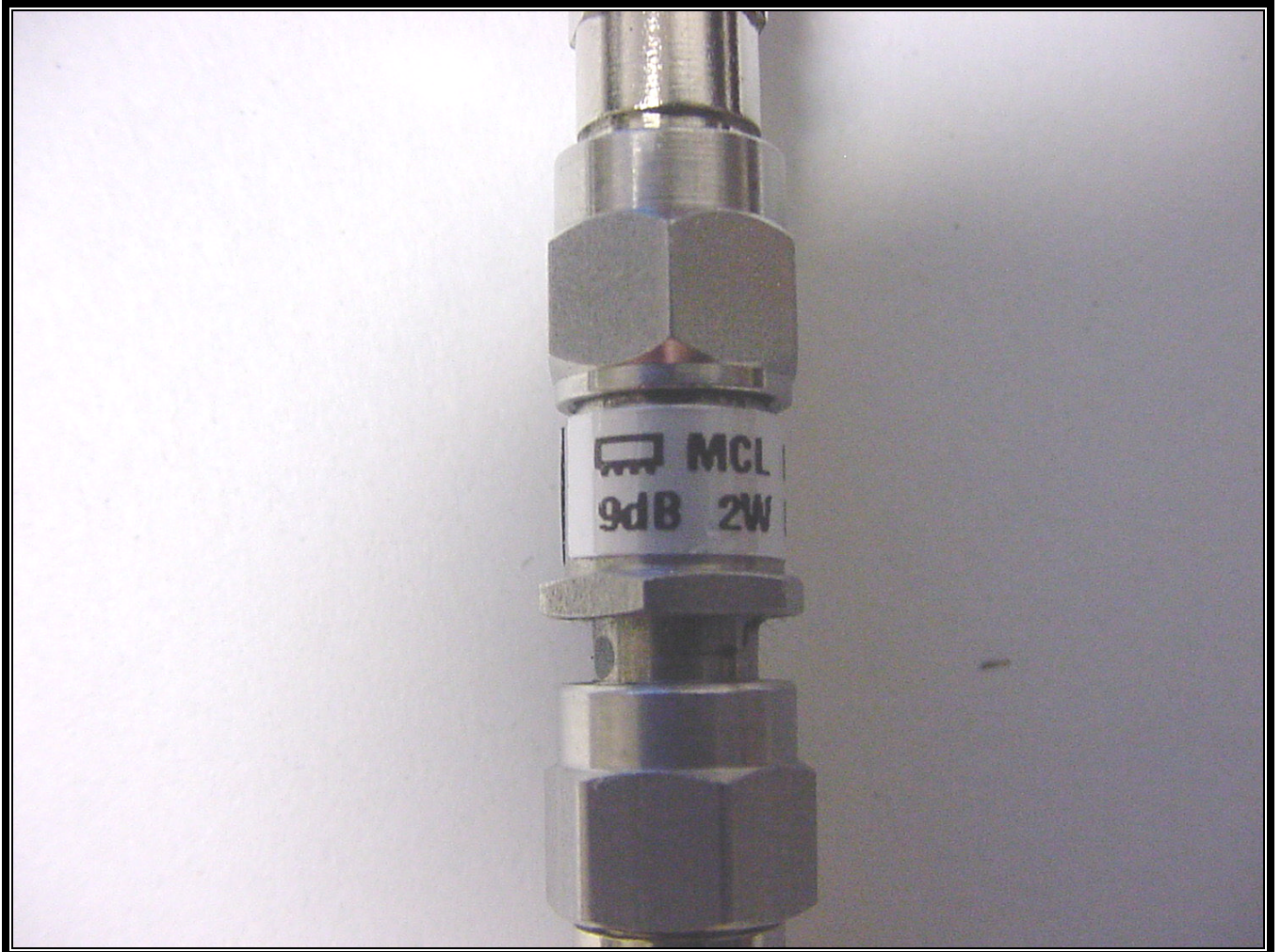
PHOTOGRAPH 13: INLINE WITH ANTENNA SMA 9 DB ATTENUATOR
